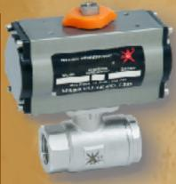
No bracket and adapter are required, the valve stem is an integral part of the actuator drive. The direct valve stem coupling to actuator shaft ensures correct alignment of the valve to the actuator, minimizes stem side loading and backlash during operation, increased service life and performance.
